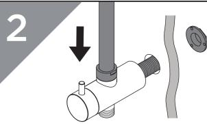
Connect the water supply to the diverter inlet and secure to the wall. Screw the riser rail into the top of the diverter.
