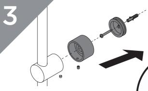
Remove the wall bracket fixing.
