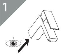
Look underneath the tap body to observe fixing kit rod(s) and tail inlet positions
