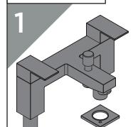
Feed the tap body through the plinths and ensure rubber plinth seals are in place
