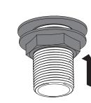
To secure the taps to the bath, use a box spanner to tighten the metal backnuts underneath ensuring the washer is correctly positioned in between the backnuts and the bath
